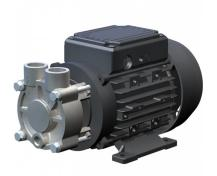
These non-self-priming or self-priming regenerative turbine pumps are characterised by their high pressure with low flow rates and their compact construction. They can be applied in circuits for liquids not containing solid matter, for example in temperature control units or machine cooling systems, among others.
